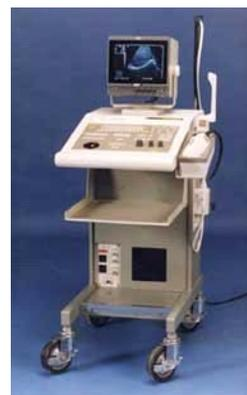
Ultrasound scanners consist of a console containing a computer and electronics, a video display screen and a transducer that is used to scan the body. The transducer is a small hand-held device that resembles a microphone, attached to the scanner by a cord. The transducer sends out a high frequency sound wave and then listens for a returning sound wave or "echo".
